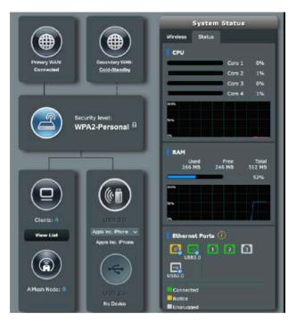
You can monitor the CPU status of each core, the RAM usage status and the Ethernet ports status. The following is an example of the CPU, RAM and Ethernet ports usage status.
